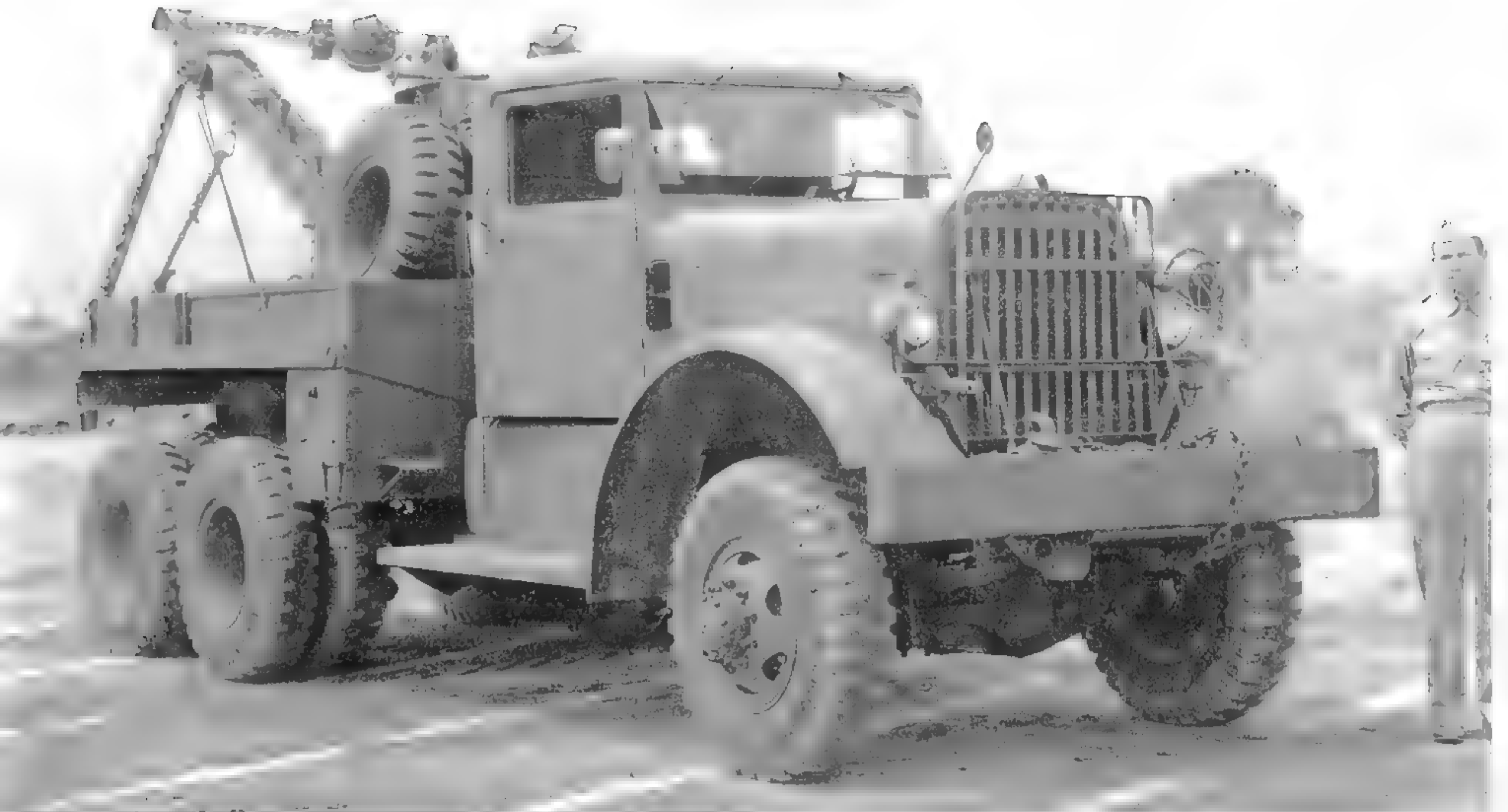
This June 1942 Aberdeen Proving Ground photo shows the first Kenworth-produced M1 wrecker. Known by Kenworth as the model 570, II was almost identical to the Ward LaFrance Series 2 trucks, although there were some differences in control linkages. (NARA photo)
